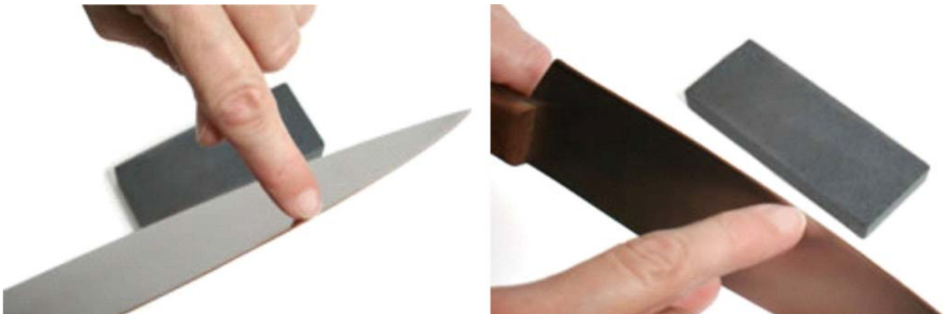
Figure 14 Checking the Bevelled Edge
